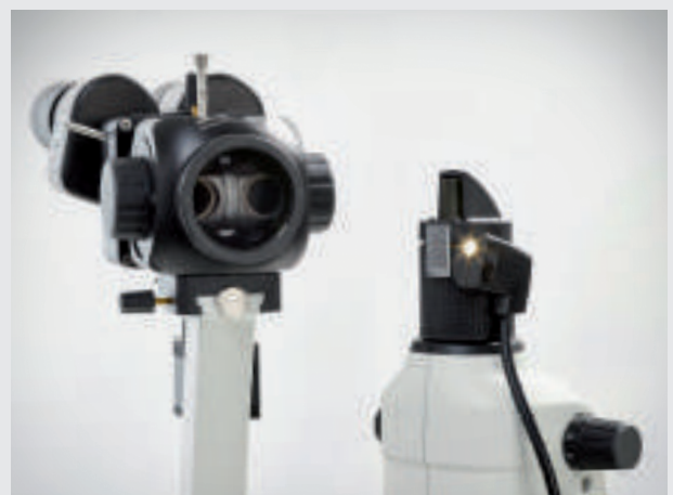
Background illumination system of the SL-IC4 D
